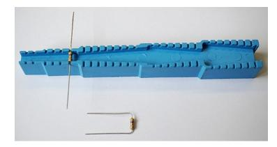
The bending tool, see picture above, is a very handy tool to make a perfect fit. The PCB has exact this distances.
