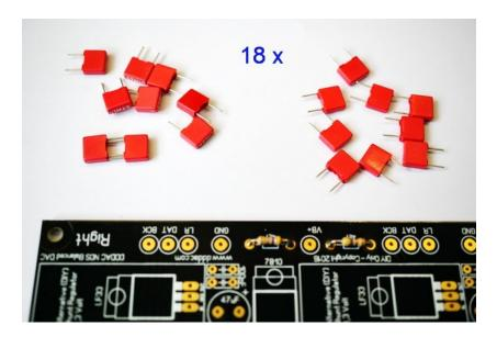
Next we will solder the 18 pcs of the 100nF capacitors. Best is to put them on the pcb and slightly bend the two wires to the outside so they will not fall off the board anymore.
