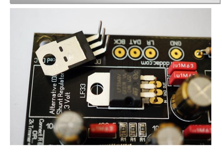
Press the connection pins through the PCB. Solder the middle pin with a small drop while making sure the voltage regulator is nicely placed on the PCB. (See image).
