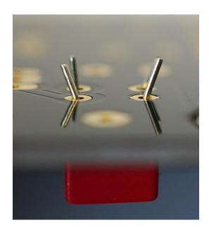
Place the PCB on its back on a flat working space. Make sure all capacitors are placed correctly. Press slightly to make sure this is the case. Now solder all 36 connections. Cut them short with the cable cutter.
