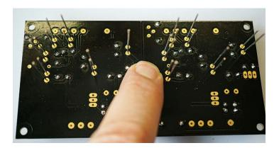
Again, take your time to let the solder flow. Specially the "minus" poles are at the ground plane which will attract quite some heat in the first few seconds when the solder tip is placed. So do not "bake" the solder on the pads. Let it flow.
