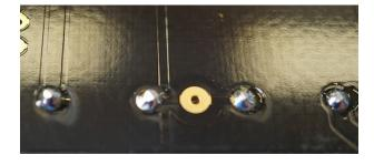
Let the solder flow nicely round the wires (must be shiny) and cut the wires with the cable cutter. Cut them directly above the solder pad.
