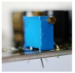
The adjusting of the CSS can only be done after the dac module is installed on the main board. The measurement control point is the solder pad directly next to the trimmer. Here we need a DC voltage of + 40mV (hold the red 'plus' of your DMM at this point)
