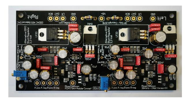
Finally!! The new, highly improved '2016' DDDAC1794 module! De voltage regulation at the analog side of the system has now an embedded Tentlabs Shunt regulator. The Bias through the much discussed 'pin 20' got a constant current source (CCS) which replaces the fixed 6K1 resistor. All resulting in the next stage of superb sound reproduction
